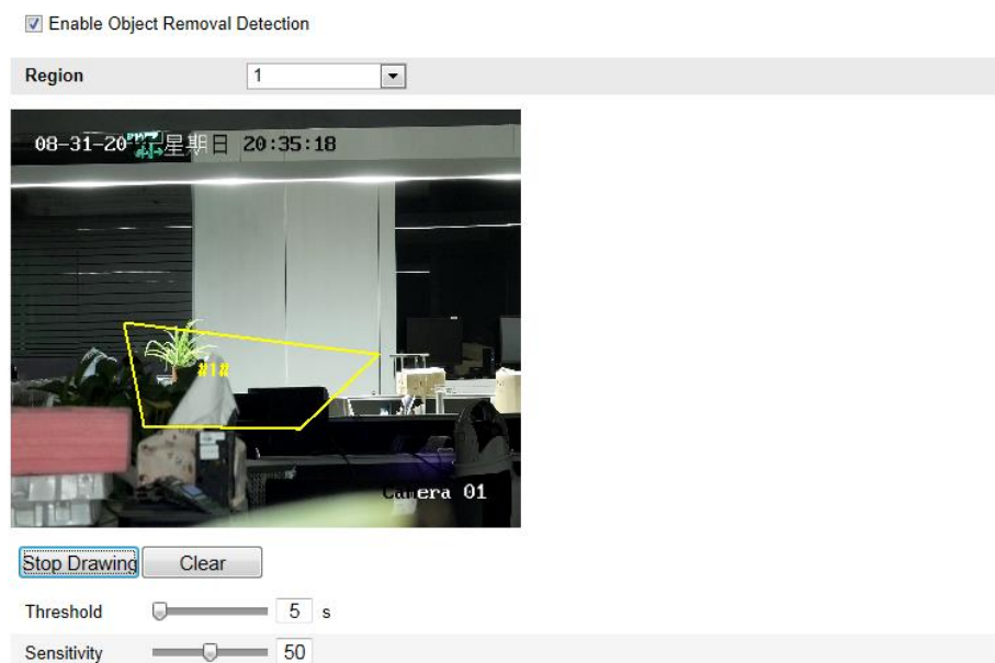
Figure 6-65 Configuring Object Removal Detection
