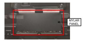
S28 Tear off "FABRIC CONDUCTIVE U" from "Panel"
