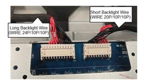
S16 Tear off 4 acetate tapes which are for covering the connectors of backlight on Panel
