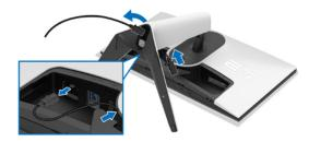
Press and hold the stand release button at the back of the display
