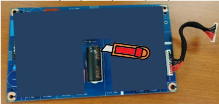
S35-2 Ensure cutting path within the glue, don't touch bulk cap. or PCB
