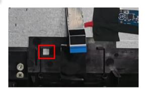
Tear off 6 acetate tapes from Backlight Wires on Panel
