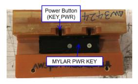
S27 Unlock 2 screws and disassemble "LENS BD" (Power LENS BD) from Power Button
