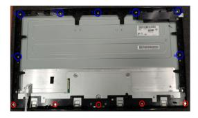
(Screw Torque-Bottom MF: 4.0±0.5 kgf) (Screw Torque-Top MF: 7±0.5 kgf)
