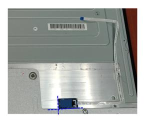
S22 Unplug "Thermal Sensor BD FFC" from "Thermal Sensor BD"
