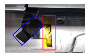
S21 Tear off "Thermal Sensor BD FFC" from Panel
