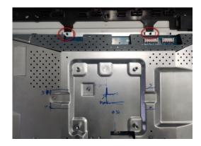
S20 Tear off an acetate tape and a yellow tape from "FFC EDP 60P/60P"
