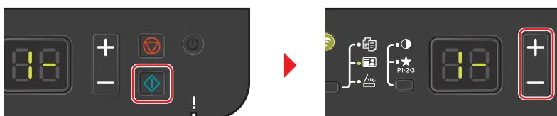
After the first side is scanned, 2– appears in the display.
