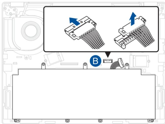
To connect the battery, align and connect the cable to the battery connector before you reattach the compartment cover.
