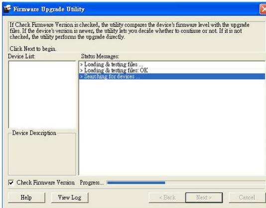
4. The Utility inspects your installation. All the devices capable of being upgraded by the package are listed in the *Select Master Device* list.
