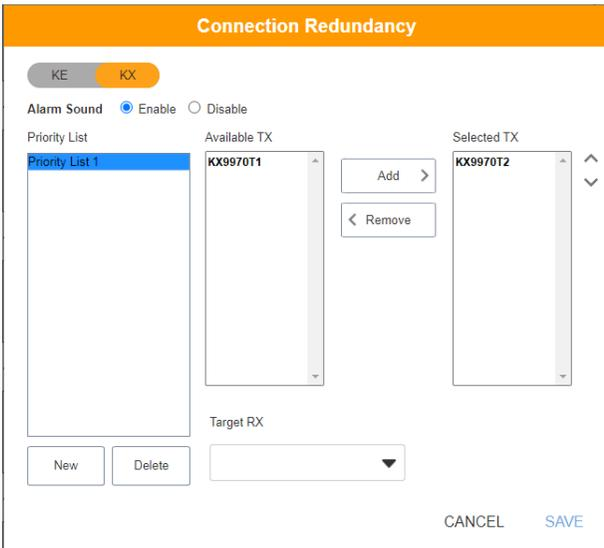
To deselect the transmitter, click to select the transmitter from the “Selected TX” list and click **Remove**. The transmitter will be shifted back to the “Available TX” list.
