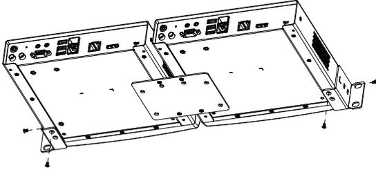
5. Screw the mounting brackets onto the rack.
