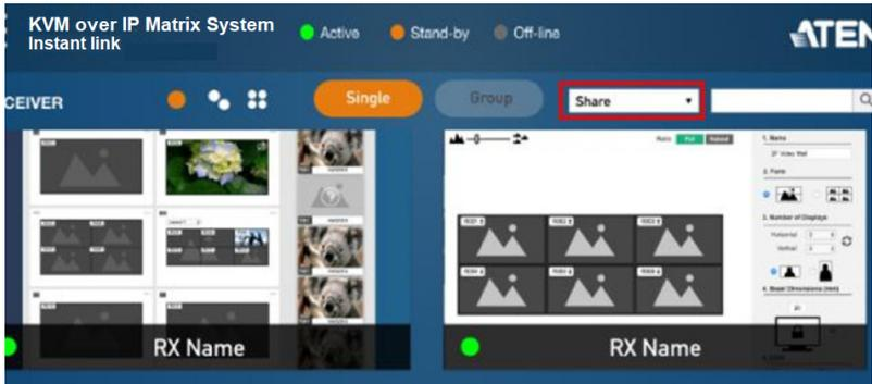
2. Tap and drag the desired transmitter device or Tx group to the desired receiver or Rx group, as illustrated below.
