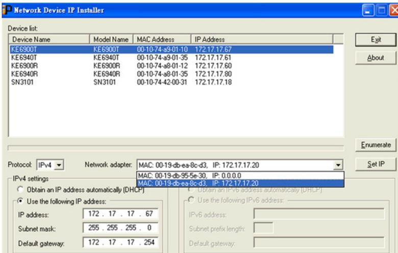
3. Select the Transmitter or Receiver in the Device List.
