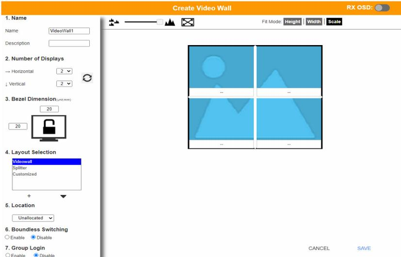
Select the number of displays and then group multiple displays to form large screens and/or use single displays for independent screens to create the video wall's layout. Click the bar -- under the display icon to select a Receiver for each display. This configuration should match the actual video wall layout.
