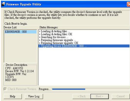
If you enabled *Check Firmware Version*, the Utility compares the device's firmware level with that of the upgrade files. If it finds that the device's version is higher than the upgrade version, it brings up a dialog box informing you of the situation and gives you the option to **Continue** or **Cancel**.
