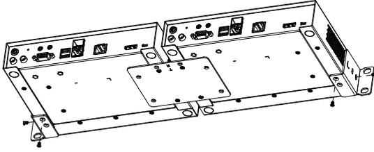
4. Screw the mounting brackets onto the rack.
