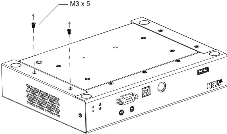
2. Use the screws from step 1 to attach the mounting bracket to the bottom of the transmitter, as shown below.
