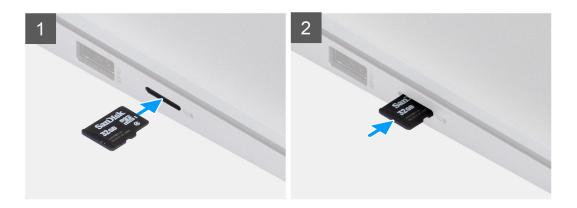
Insert the micro-SD card into its slot until it clicks into place.
