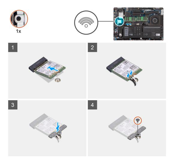
Connect the antenna cables to the WLAN card.
