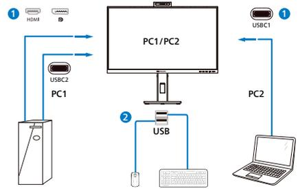
3. Enter to OSD menu. Go to KVM layer and select "Auto", "USB C1" or "USB C2" to switch the control of peripherals from one device to another. Simply repeat this step for switching the control system using one set of peripheral.
