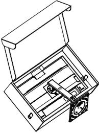
2. Place the monitor face down on a smooth surface. Pay attention not to scratch or damage the screen. Then lift the monitor stand.
