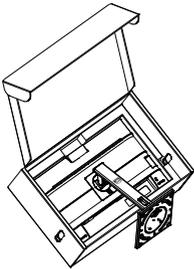
3. While keeping the release button pressed, tilt the base and slide it out.
