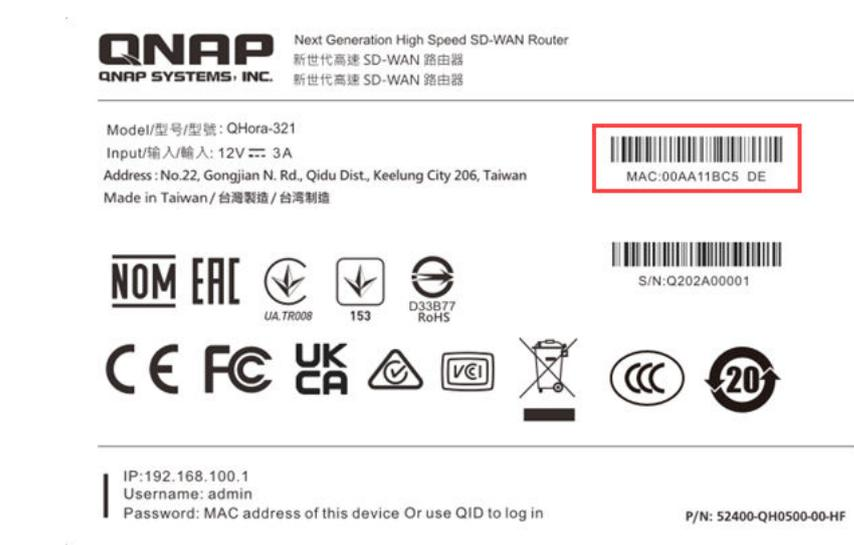
The MAC address can be found on the asset tag on the bottom of the device.
