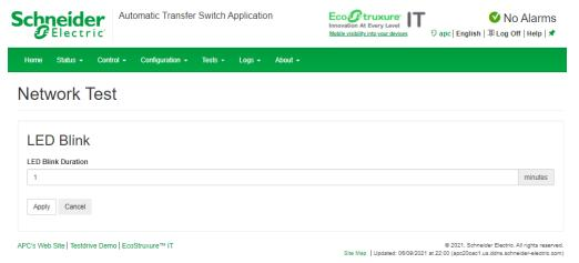
If you are having trouble finding your Rack ATS, enter a number of minutes in the **LED Blink Duration** field, and click **Apply**. The 10/100/1000 Status LED light on the display will blink for the specified number of minutes.
