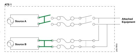
Two or four non-replaceable fuses (depending on the model) help to protect the Rack ATS from short circuits (ATS 2).
