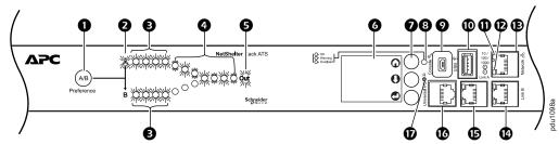
Your Rack ATS is configured so the display backlight turns off after 10 minutes of inactivity. Press any display navigation button to illuminate the backlight.
