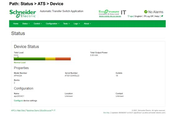
View the **Device Status**, **Properties**, and **Configuration** information. Select **Configure device settings** to edit the **Name**, **Location**, or **Contact** information.
