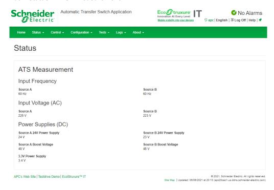
View measurements for Input Frequency, Input Voltage (AC), and Power Supplies (DC).
