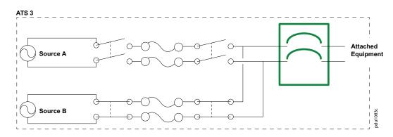
The Rack ATS does not include power surge protection. To help protect your Rack ATS from external power surges, it is recommended that you always connect each Rack ATS source to a Double Conversion On-Line Uninterruptible Power Supply (UPS).
