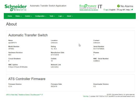
The hardware information is useful to APC Customer Support for troubleshooting problems with the Rack ATS. The serial number and MAC address are also available on the Rack ATS itself.
