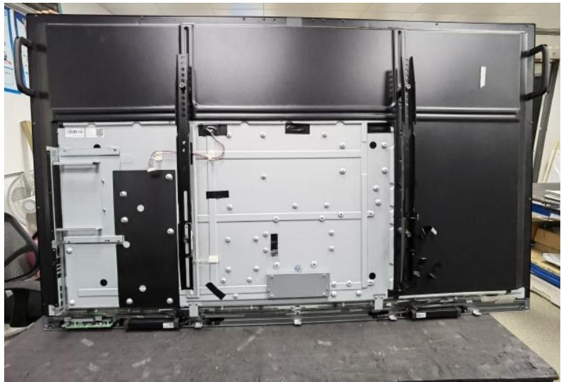
1、 Use an electric screwdriver to remove the fixing screw of the glass pressing block and remove the glass pressing block.
