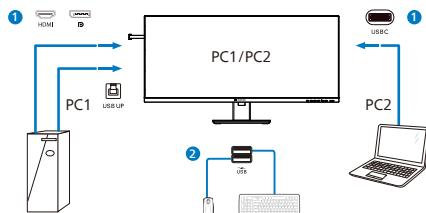
3. Enter to OSD menu. Go to KVM layer and select "Auto", "USB C" or "USB up" to switch the control of peripherals from one device to another. Simply repeat this step for switching the control system using one set of peripheral.
