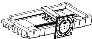
2. Loosen the assembly screws, then detach the neck from the monitor.
