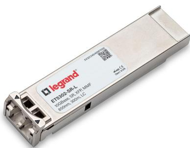
Edgecore ET5302-SR Compatible 10GBase-SR XFP Transceiver (MMF, 850nm, 300m, LC Duplex, DDM, I-Temp)
