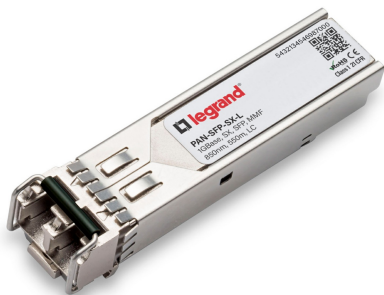
Palo Alto PAN-SFP-SX Compatible 1000Base-SX SFP Transceiver (MMF, 850nm, 550m, LC Duplex, DDM, I-Temp)
