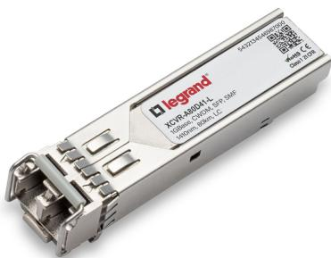
Ciena XCVR-A80D41 Compatible 1000Base-CWDM SFP Transceiver (SMF, 1410nm, 80km, LC Duplex, DDM, I-Temp)
