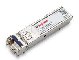
MSA SFP-BX35-40-I Compatible 1000Base-BX SFP Transceiver (SMF, Tx: 1310nm Rx: 1550nm, 40km, LC Duplex, DDM, I-Temp)
