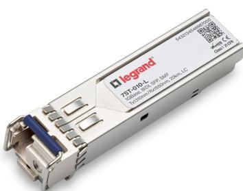
Accedian 7ST-010 Compatible 1000Base-BX SFP Transceiver (SMF, Tx: 1310nm Rx: 1550nm, 20km, LC Duplex, DDM, I-Temp)
