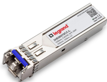
Nokia 3HE00070CC Compatible 1000Base-CWDM SFP Transceiver (SMF, 1510nm, 120km, LC Duplex, DDM, I-Temp)
