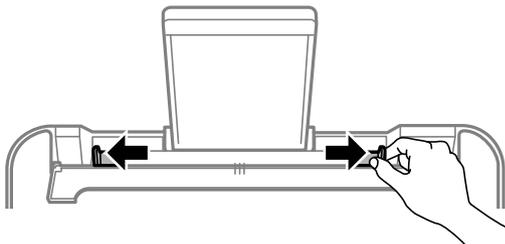
3. Load envelopes short edge first at the center of the paper support with the flap facing down.
