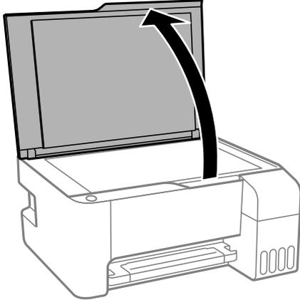
2. Remove any dust or stains on the surface of the scanner glass using a soft, dry, clean cloth.
