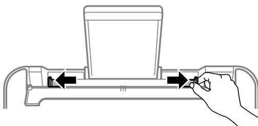
3. Load paper at the center of the paper support with the printable side facing up.
