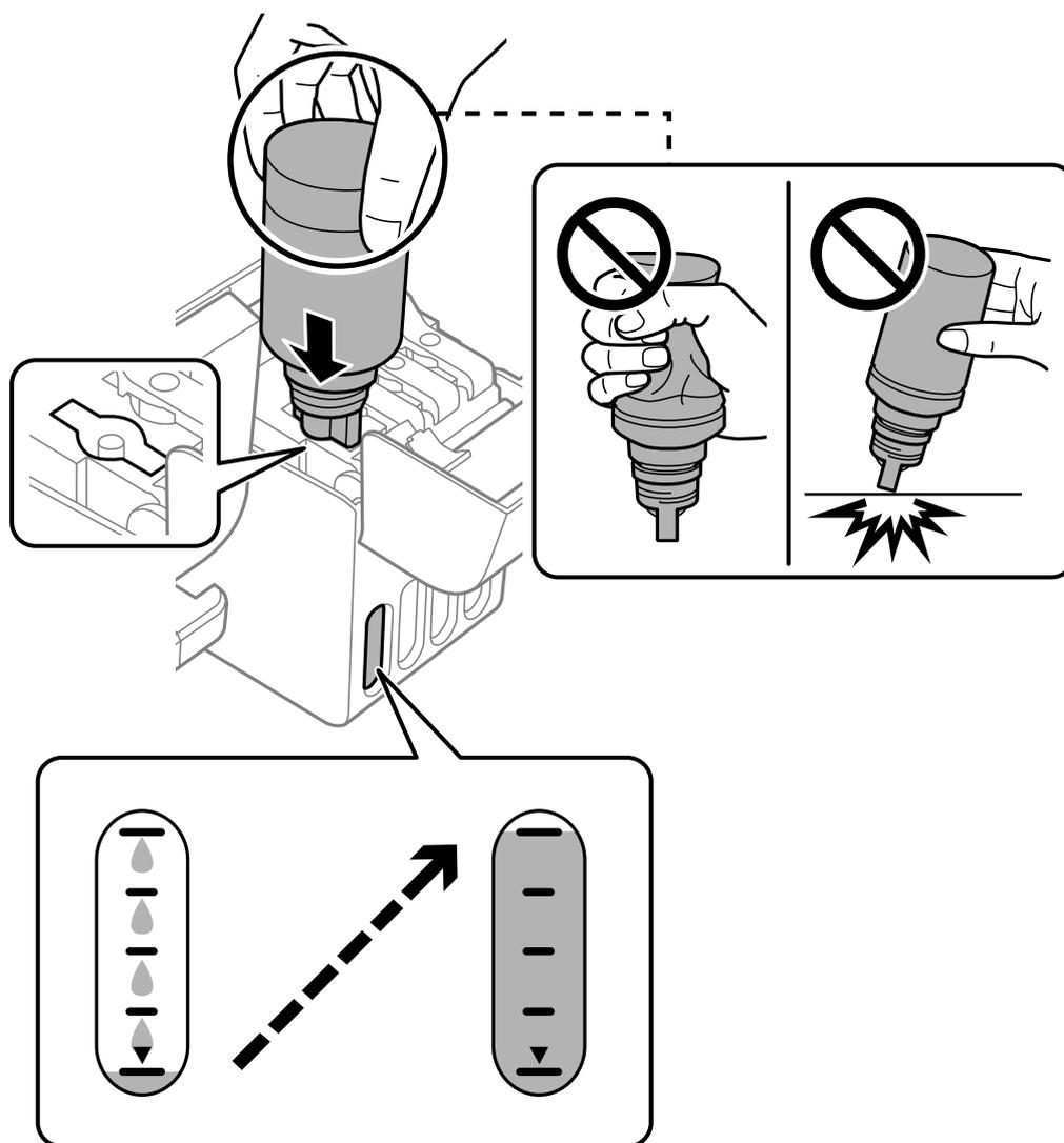
6. When you have finished refilling the ink, remove the ink bottle, and then close the ink tank cap securely.
