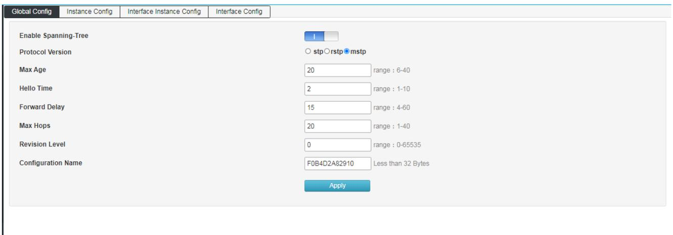
Use Enable Spanning-tree to turn spanning tree on/off
