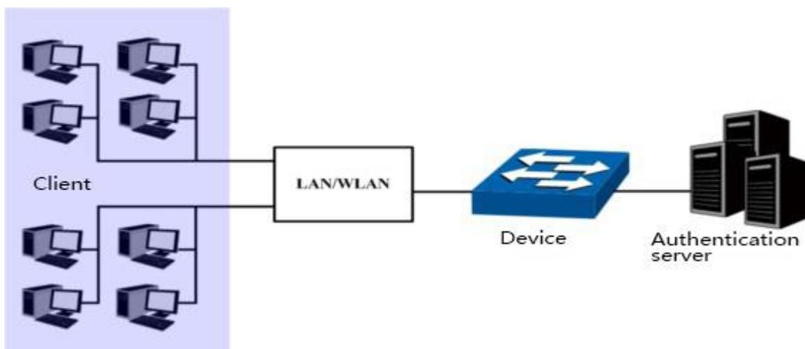
1) Client: An entity in the LAN, mostly an ordinary computer. The user initiates 802.1X authentication through the client software and is authenticated by the device. The client software must be a user terminal device that supports 802.1X authentication.
