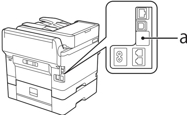
2. Connect the USB cable for the authentication device to the service port.
