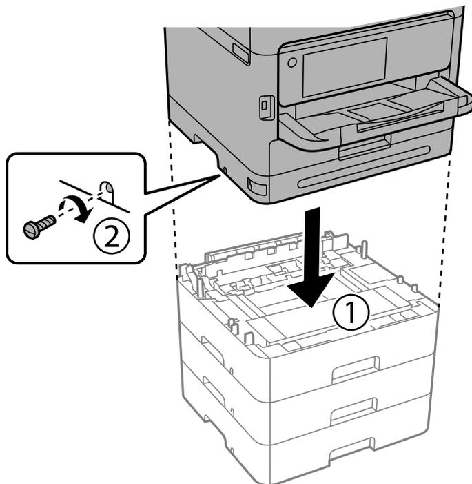
12. Secure the optional paper cassette units and the printer at the back and the right side with the screws using a screwdriver.
