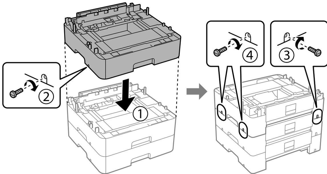
11. Lower the printer gently onto the optional paper cassette units aligning the corners, and then secure them with the screws using a screwdriver.
