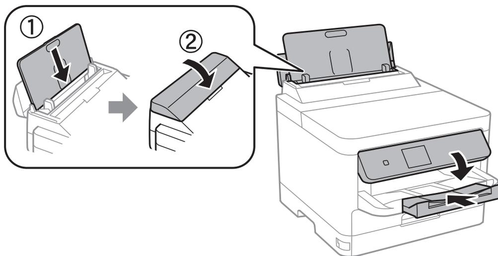
13. Remove the output tray from the printer.
