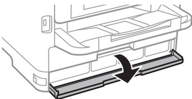
If the ink cover is locked, you cannot open it. Release the cover lock.
