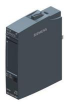
SIPLUS ET 200SP RQ 4x24VUC/2A ST TX rail based on 6ES7132-6GD51-0BA0 with conformal coating, -40...+70 °C, OT4 with ST1/2 (+85 °C for 10 minutes), signal relay module, suitable for BU type A0, color code CC00, substitute value output, module diagnostics for: supply voltage
