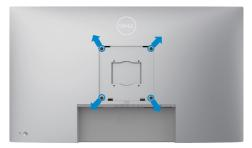
NOTE: Use M6 x 35 mm (200 mm x 200 mm) or M4 x 12 mm (100 mm x 100 mm) screws to connect the monitor to the wall-mounting kit.
