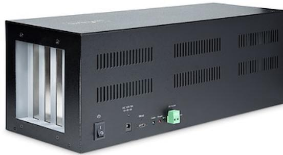
The robust expansion chassis supports 4 PCIe x1 add-on cards and features up to 10Gbps of total bandwidth. The expansion chassis connects to the host using a proprietary USB-C PCIe x2 adapter card and a locking USB Type-C cable. Take advantage of features such as Wake-on-LAN (WoL), support for PCI Express Advanced Error Reporting (AER), backwards compatibility, and multiple power capabilities.
