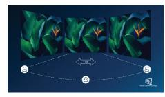
IPS displays use an advanced technology that gives you extra-wide viewing angles of 178/178 degrees, making it possible to view the display from almost any angle. Unlike standard
