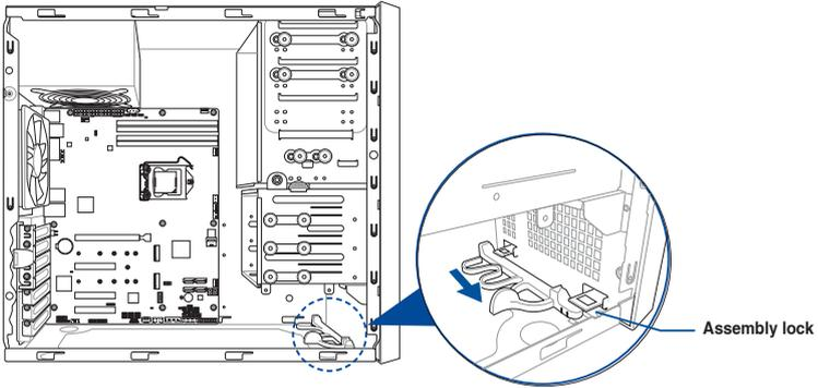
2. Remove the front panel assembly from the chassis and set it aside.
