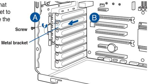
4. Align and insert the expansion card into the PCIe slot.
