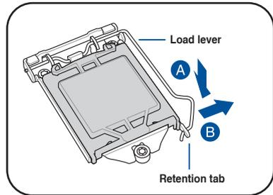
2. Lift the load lever until the load plate is completely lifted.
