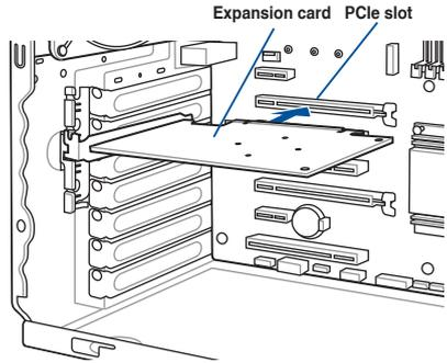
5. Lift the PCIe latch inwards until it clicks into place securing the expansion card to the chassis.
