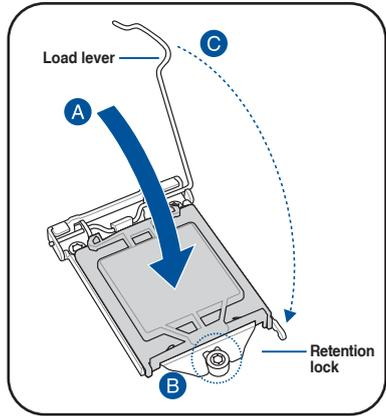
5. Insert the load lever under the retention tab to remove the PnP cap from the CPU socket.
