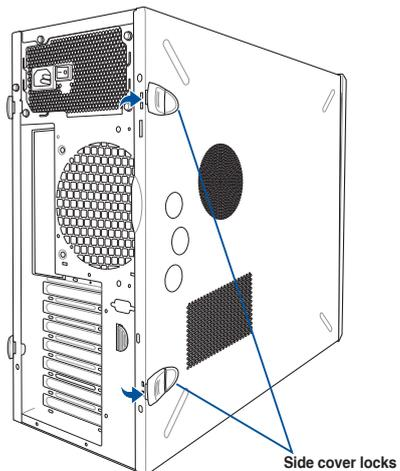
3. Slightly pull the side cover toward the rear just enough to detach it from the chassis.
