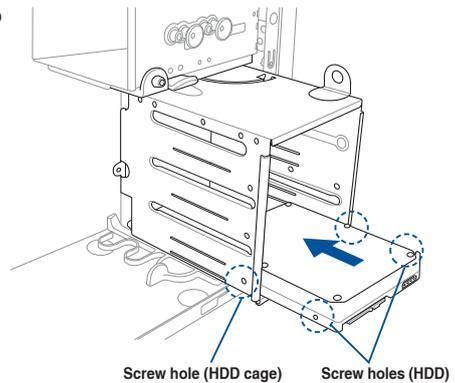
5. Secure the 3.5-inch HDD to the HDD cage using the bundled set of screws.
