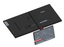
Step 3: Remove the base and stand from the monitor, refer to "Detaching the monitor base and stand" on page 2-11.
