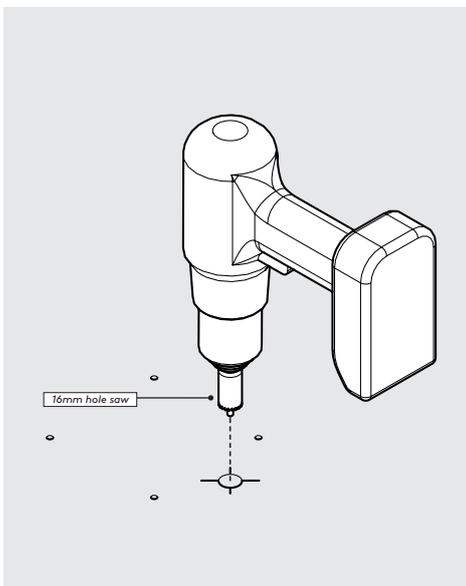
**A3** If running a ethernet or USB cable through the surface use a hole saw in the cable exit position.
