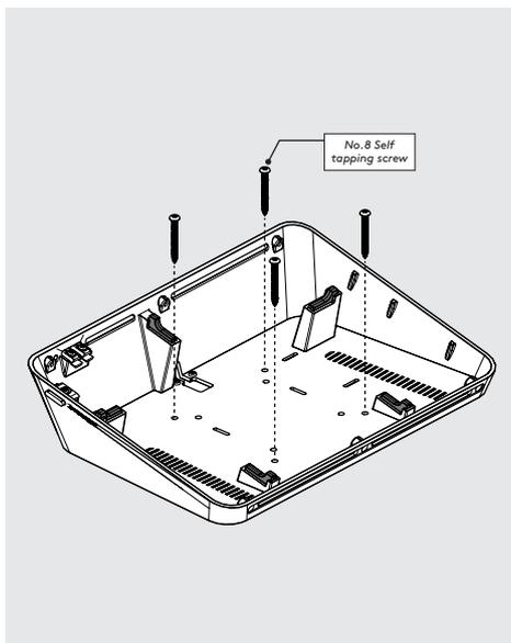
**A4** Secure the Link to the surface with 4x No.8 Self tapping screws. Rawl plugs are provided if required.
