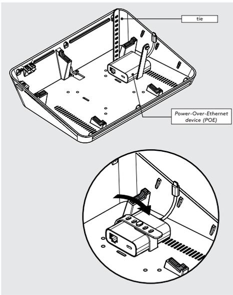
**5** Insert the tie through the cable slots and then clasp over the POE device.
