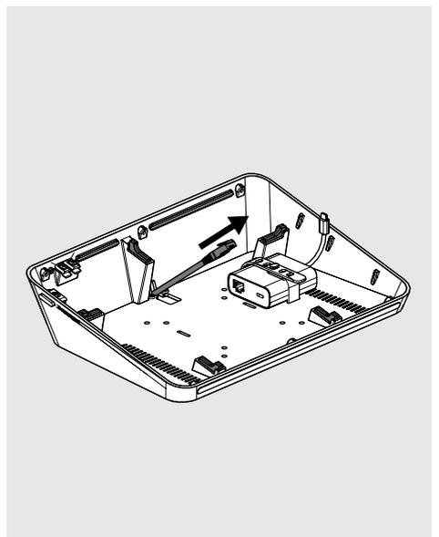
**7** Feed the ethernet cable through the cable exit.
