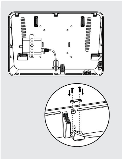
**8** Connect the ethernet cable to the POE and secure the cable with the cable lock.
