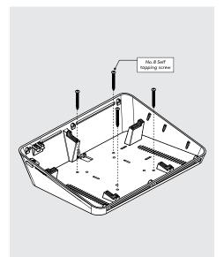
Secure the Link to the surface with 4x No.8 Self tapping screws. Rawl plugs are provided if required.
