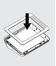
Connect the USB cable to the tablet, then place inside the enclosure. Reattach the faceplate.
