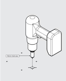
If running a ethernet or USB cable through the surface use a hole saw in the cable exit position.
