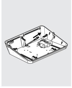
Insert the tie through the cable slots and then clasp over the POE device.
