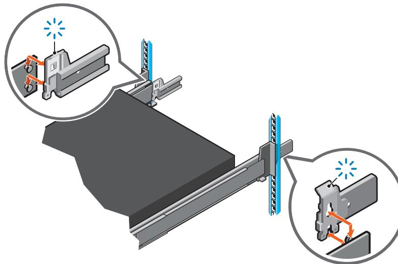
**NOTE:** The SRB has two positions for various rack environments
