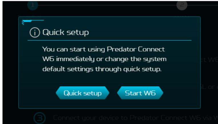
1. If this is the first time you are using or setting up the Predator Connect W6 Wi-Fi 6E Router, please proceed by clicking the “Quick setup” button.
