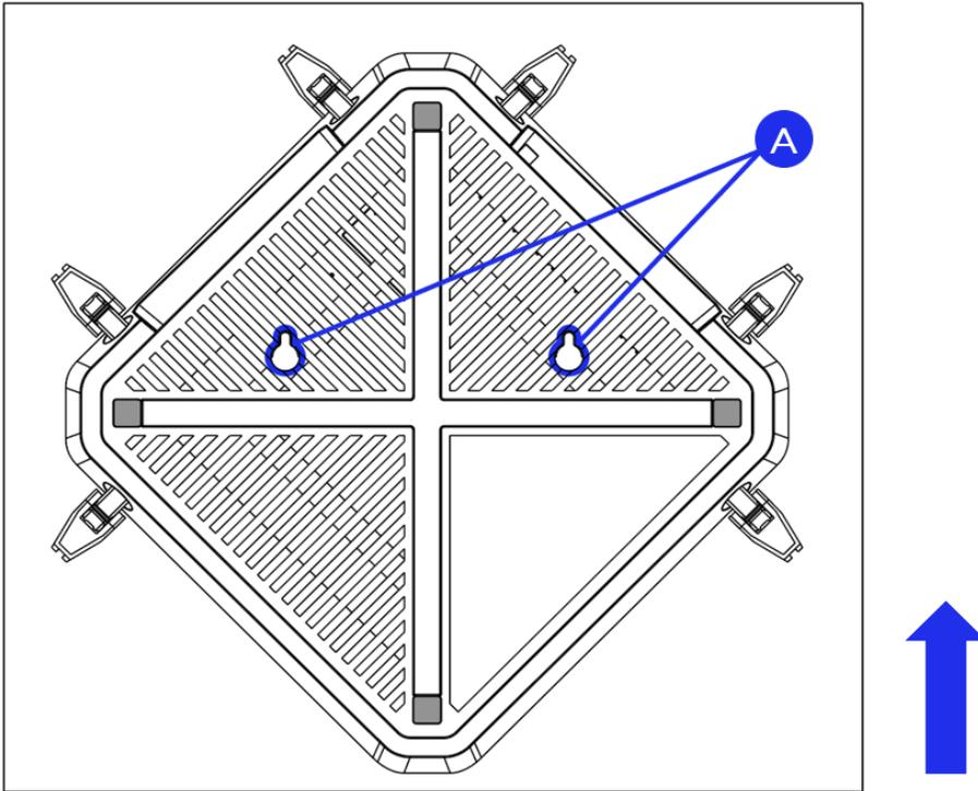
A: 2 Wall Mount Holes in blue outlines at 10cm or 4inches wide. Follow the reference image above for correct orientation and proper device mounting.
