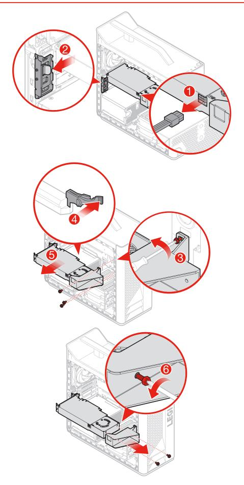
**NOTE:** When you install the PCI express adapter, place the PCI port area toward the EMI gasket with the correct orientation.
