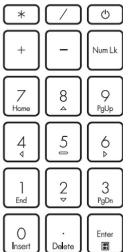
A numeric keypad is available on selected Notebook PC models. You can use this keypad for numeric input or as pointer direction keys.
