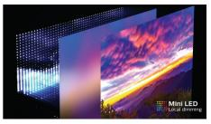
Mini LED backlighting improves control of lighting and contrast ratio. The small size of the mini LEDs forming the backlight allows for the creation of 1152 individually controlled zones delivering deeper blacks and brighter whites. Rich HDR content can now be viewed as it was intended with unmatched contrast and precise reproduction.
