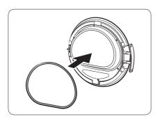
7. Insert the door sealing in the correct position.
