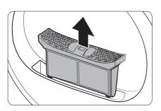
1. Open the door and pull the lint filter upward to remove.
