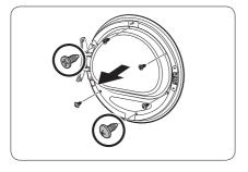
**3.** Remove the upper 3 screws and the lower 3 screws on the glass holder.
