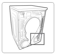
The dryer comes with a built-in water tank. However, if you do not want to use the water tank, you may install the drain hose. The provided accessory hose (long drain hose) can be used as an extension to the drain hose.
