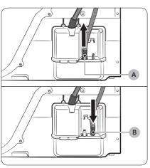
1. Remove the drain hose from hole (A), and insert it into hole (B).
