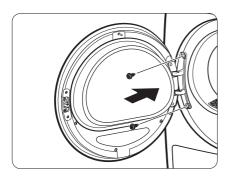
**12.** Put the door hinge on the opposite side, and then tighten the 2 screws to fix the door to the dryer.
