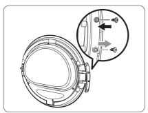
**11.** Remove the screw on the bottom of the door hinge, and the fasten it on the top of the door hinge.
