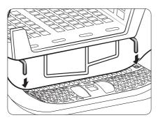
1. Position the drying rack in the drum, inserting the front lips of the rack into the holes of the door diaphragm.
