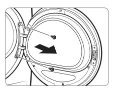
1. Open the door, and then remove the two screws on the door hinge. While holding the door with both hands, slightly lift to remove it.
