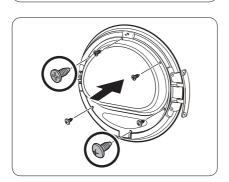
**6.** Tighten the upper 3 screws and the lower 3 screws on the glass holder.
