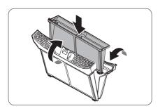
**5.** Put the inner filter into the outer filter, and then reinsert the lint filter into the original position.
