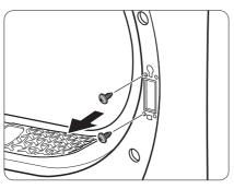
8. Remove the 2 screws that remain after removing the door hinge.
