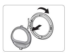
**4.** Remove the glass holder, and then rotate the door cover by 180 degrees.
