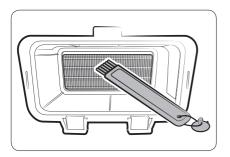
4. Clean the heat exchanger with the provided cleaning brush or a vacuum cleaner with a brush attachment. Take care not to bend or damage the heat exchanger fins when cleaning. This may lead to a decrease in drying performance.
