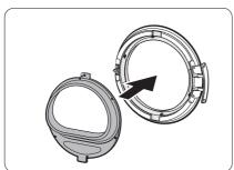
**5.** Insert the glass holder into the new position of the door cover. Make sure the door hinge is in the same position as in the figure.
