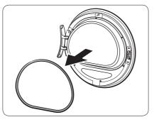
**2.** Use a thin object to remove the door sealing.
