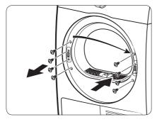
9. Remove the 4 screws on the door lock. Remove the door lock, and then reinsert it to the opposite side.
