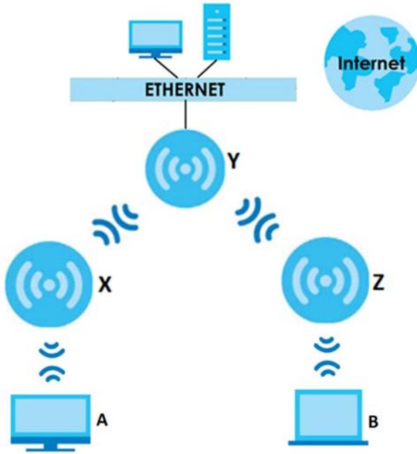
The Zyxel Device can also serve as a wireless bridge in Repeater mode. A wireless bridge connects two wired networks through a wireless connection. When the Zyxel Device is connected to a root AP, enable wireless bridge to allow traffic through the Ethernet port on the Zyxel Device to a wired network. Check [Section 1.2 on page 13](#) for models that support wireless bridge.
