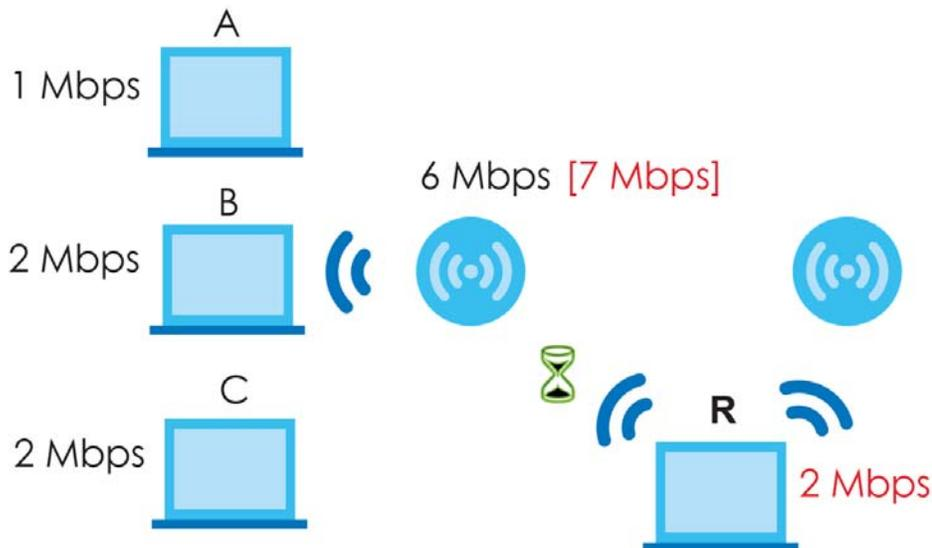
The second response your AP can take is to disassociate with clients that are pushing it over its balanced bandwidth allotment.
