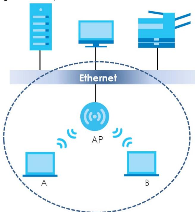
The WiFi network is the part in the blue circle. In this WiFi network, devices **A** and **B** are called WiFi clients. The WiFi clients use the access point (AP) to interact with other devices (such as the printer) or with the Internet. Your Zyxel Device is the AP.
