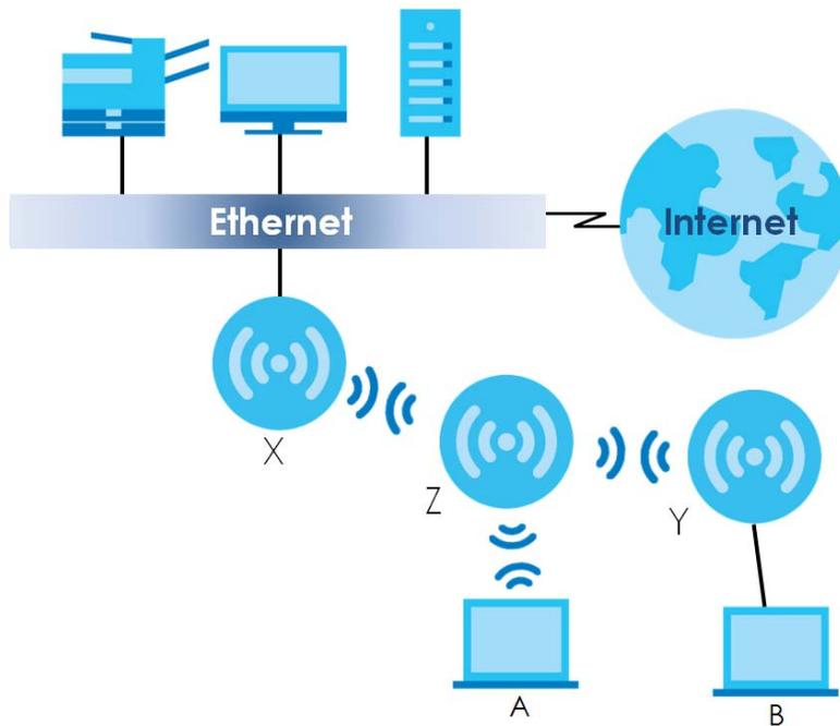
When the Zyxel Device is in Repeater mode, repeater security between the Zyxel Device and other repeater is independent of the security between the WiFi clients and the AP or repeater. When repeater security is enabled, both APs and repeaters must use the same pre-shared key. See [Section 10.2 on page 95](#) and [Section 14.2 on page 164](#) for more details.
