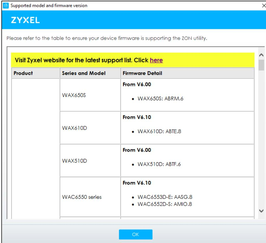
If you want to check the supported models and firmware versions later, you can click the **Show information about ZON** icon in the upper right hand corner of the screen. Then select the **Supported model and firmware version** link. If your device is not listed here, see the device release notes for ZON Utility support. The release notes are in the firmware zip file on the Zyxel web site.
