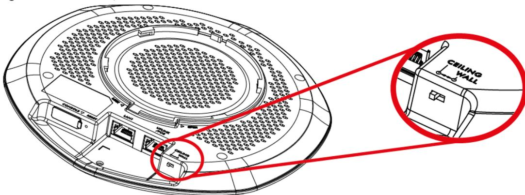
Note: With the physical antenna switch, you apply the same antenna orientation settings to both radios. You can set the radios to have different settings while using the Web Configurator or the command line interface.
