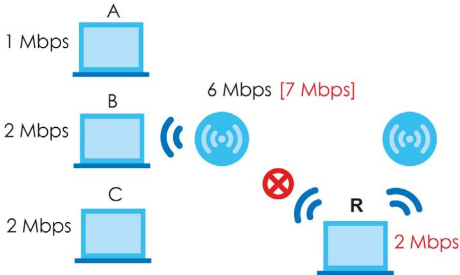
Connections are cut based on either **idle timeout** or **signal strength**. The Zyxel Device first looks to see which devices have been idle the longest, then starts kicking them in order of highest idle time. If no connections are idle, the next criteria the Zyxel Device analyzes is signal strength. Devices with the weakest signal strength are kicked first.
