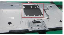
Use a Philips-head screwdriver to remove 8 screws for remove the Power board. (No.1~8 screw size=P3x4; Torque=4±1kgf.cm)
