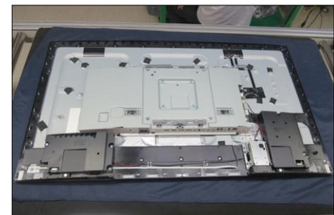
**S7** Use a Philips-head screwdriver to remove 2pcs screw for unlocking the key board, then tear off the tapes and release the key board.
