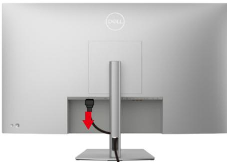
**S3** Remove stand from the product.(Press the stand release button, lift the stand up and away from the monitor)
