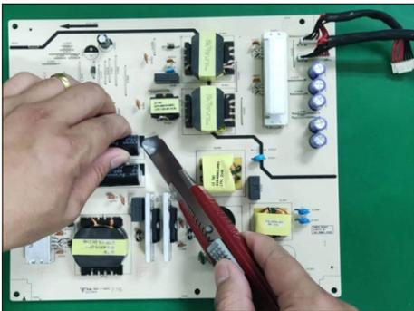
S20-3 Cut into the bottom of bulk cap. and pullit up carefully.
