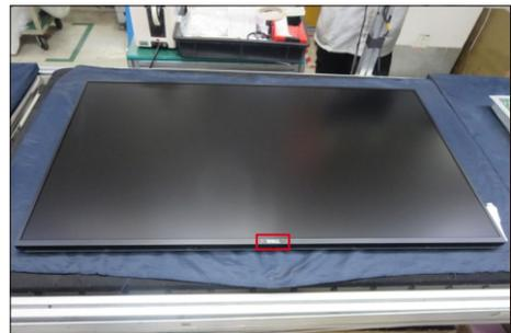
Turn over the panel module to place screen faced down. Paste 2pcs shading tape on the left and right side of the panel corner, then paste 27pcs acetate tapes on the specific position of the back of panel as the picture below shown.
