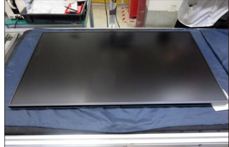
Take 1pcs Dell nameplate, then use a locating fixture to fix the nameplate to the front bezel of the module, and then move the whole unit into a laminating fixture, use the laminating fixture to press the nameplate with the bottom side of the panel module firmly attachment.
