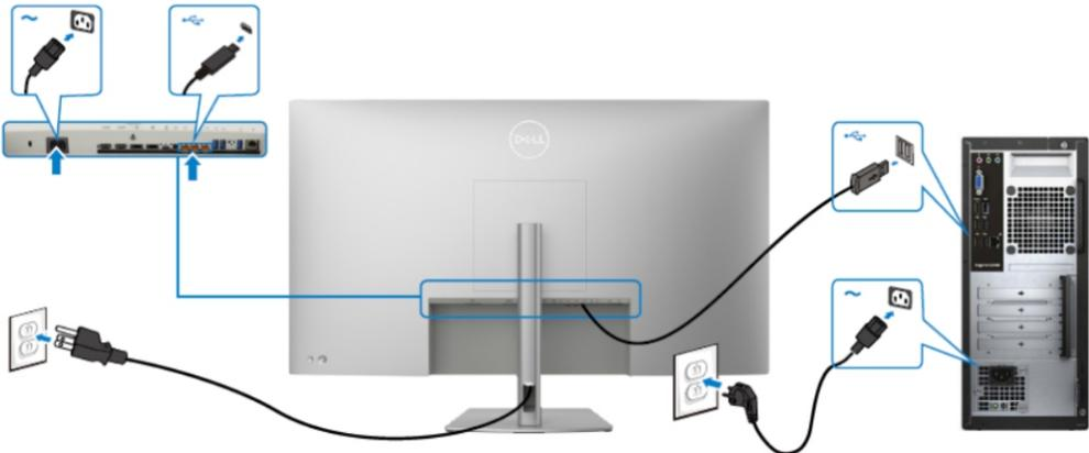
Connecting the USB-C Cable (C to C)
