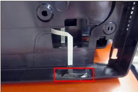
Assemble the middle frame with the panel unit, then tear off 3pcs adhesive tape papers on the back of cable and fix the LED cable on the middle frame as the picture below shown.
