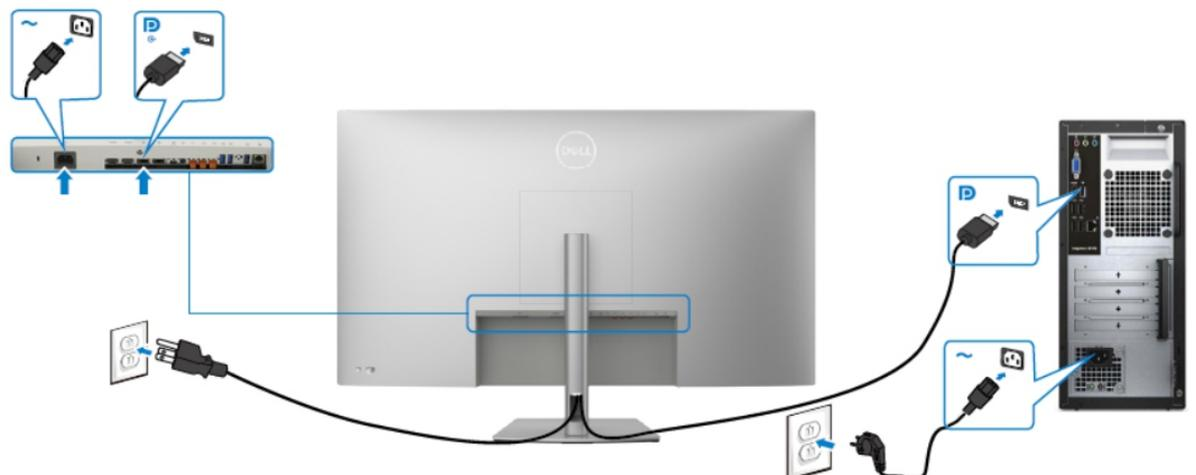
4. How to connect and disconnect power cable/ connectivity cable
