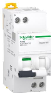
**Residual current breaker with overcurrent protection (RCBO), Acti9 iCV40H, 1P+N, 16A, C curve, 10000A, A type, 30mA**
