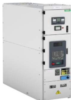
Cubicle, MCSet 17,5kV, up to 17,5kV, 31,5kA, 2500A, coupler right or left SF6 or vacuum CB 900mm
