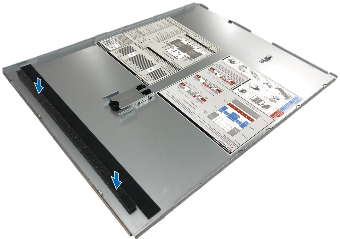
Figure 1. Installing Mylar foam on the system cover
