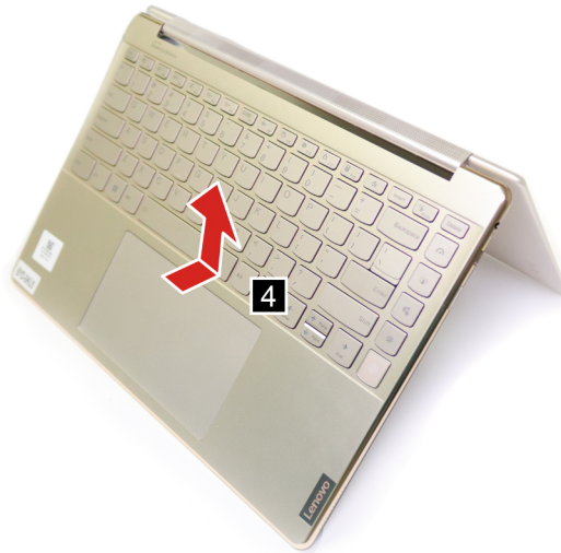
Figure 19. Remove the upper case (with keyboard)
