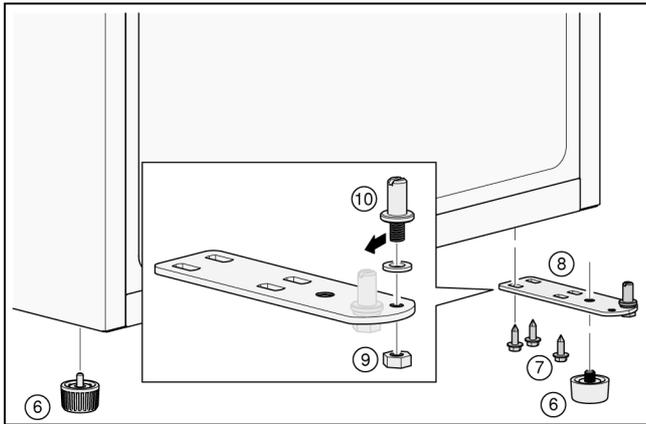
13. Insert the bolt (10) into the left boring and apply the nut (9) and tighten.
