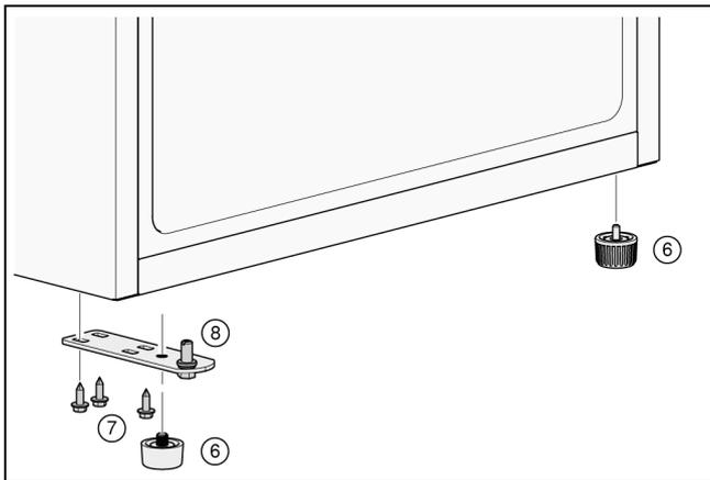
16. Attach the appliance door to the bottom hinge (8).
