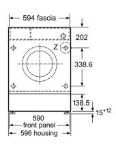
measurements in mm
