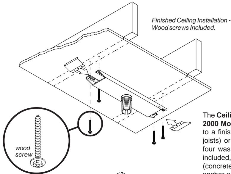
The Ceiling Plate for Jumbo 2000 Mounts can be attached to a finished ceiling (wood joists) or wood beam using the four washer head wood screws included, or a structural ceiling (concrete) using concrete anchor accessory kit ACC 204 (sold separately).
