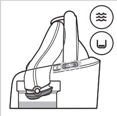
*Note: When the fluid level drops below the minimum level, the cleaning symbol and the 'fluid low' symbol start to flash with intervals and the shaver holder returns to its starting position.*
