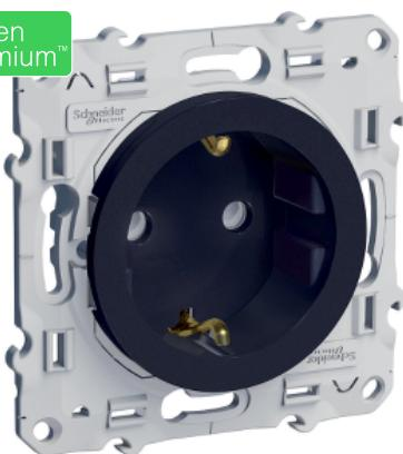
Socket-outlet, Odace, mechanism with fixing frame, 2P + E, 16A, Schuko, shutter, screwless terminals, matt, aluminium
