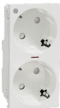
**2 Socket-outlet, New Unica, mechanism, 2P + E, 16A, Schuko, with shutter, screw terminal, glossy, antibacterial, white**
