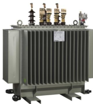
Transformer, Minera, Tier2, oil type, 160kVA, 15/20kV, 410V, 24kV
